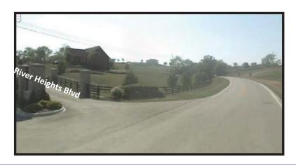
The crashes and geometry of this roadway section were investigated. There is an 8 degree curve to the right at the beginning of this segment. This is followed by a two 6 degree curves approaching River Heights Blvd. A 8 degree curve exists to the east of River Heights Blvd. Multiple curves which are in close proximity with substandard geometry are likely contributing to these crashes. The crashes recorded in this section are roadway departure crashes.
